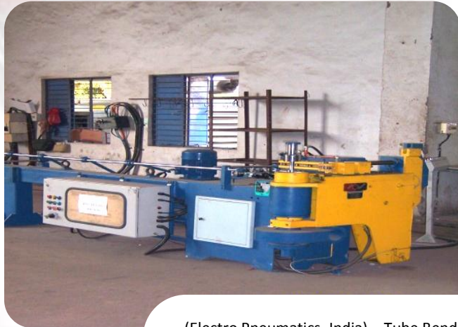
(Electro Pneumatics, India) – Tube Bending Machine 80mm x 2 mm / 65mm x 6 mm capacity.
